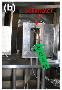
Figure 3.28: Side (a) and upstream (b) views of the collimator intended to protect the microchannel plate detector (MCP) during beam tuning. We determined that beam fragments likely scattered on the right-wall (looking from the upstream direction) of the collimator opening (See Figure 3.27.).
